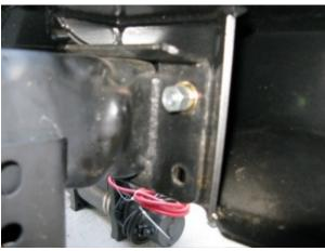
Lift Hanson bumper into place over the ends of the frame. Insert 1/2" bolt with washer from inside the bumper through the frame.
