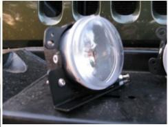
With the factory fog light removed, drill out the two tabs on the light out to 5/16". Mount using the supplied bracket and the 1/4" bolt. Complete for both lights.
