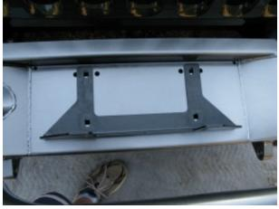
If installing a winch, the fairlead plate will mount on top of the bumper and below the winch.
