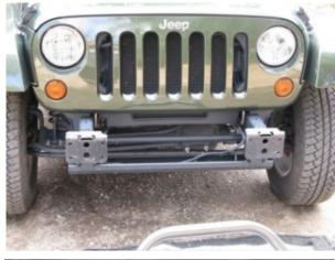
Remove stock bumper and factory valence. Also remove stock fog lights from the bumper.
