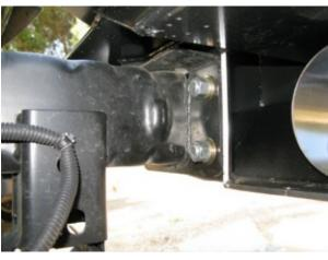
Install remaining 1/2" bolts (4 per side) and snug. Step back from the vehicle and align bumper to the Jeep. Tighten all hardware.
